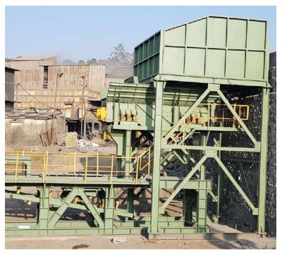
Vibration is generated by precision-machined, twin unbalanced motor. The vibrating drive assembly is connected directly to the pan to assure positive action under the most adverse loading conditions.
