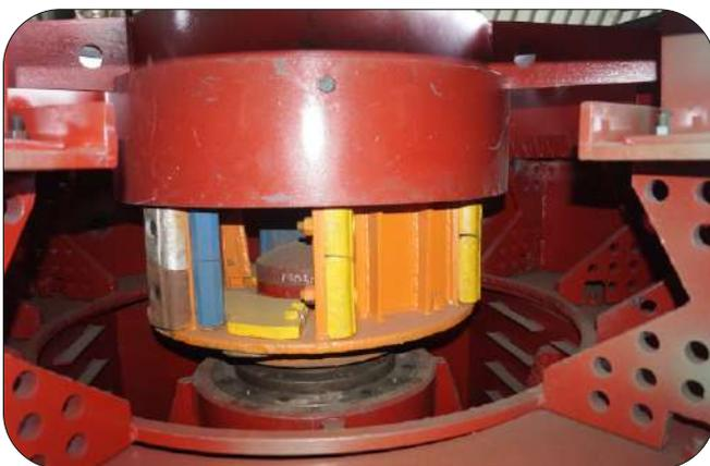
Deep chamber type rotor design perfect balance, high throughput, less wearing better versatility, easy replacement.
